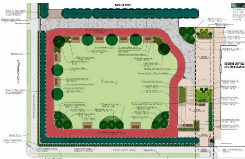
The Employee Park uses pervious paving and drought-tolerant plants.
